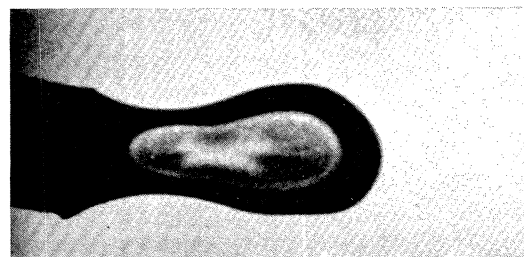
FIGURE 9 (B). Formation of stable drop of 0.18 in. diam. from stub of diameter 0.125 in. (Cine film, 750 frames/second.)
