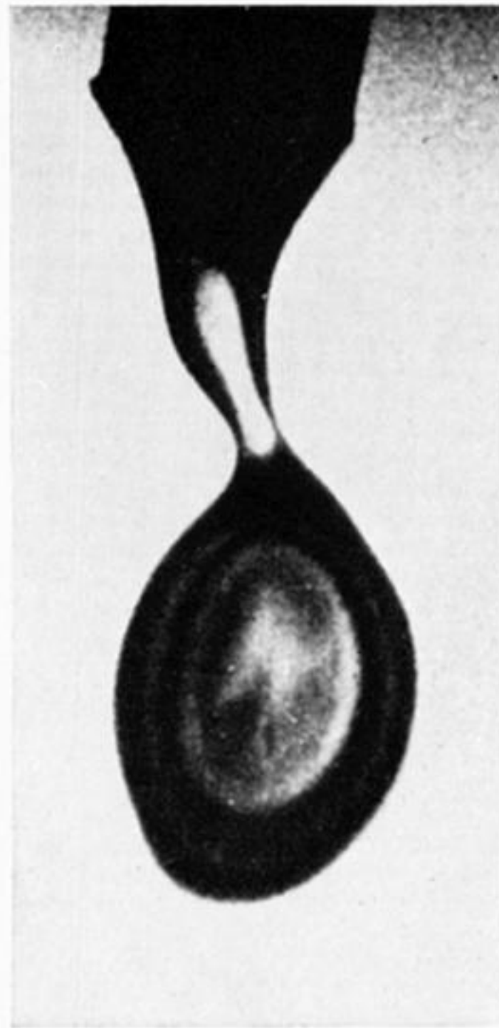
FIGURE 9 (B). Formation of stable drop of 0.18 in. diam. from stub of diameter 0.125 in. (Cine film, 750 frames/second.)
